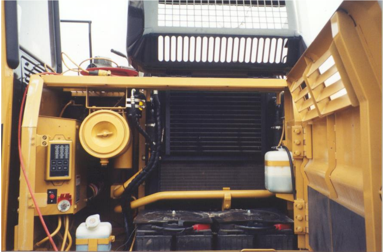
Condenser in place on 315L.
